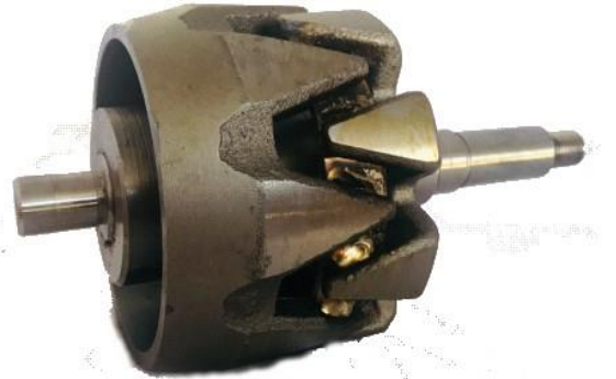
ROTOR 10510003 12V DELCO 35SI COIL 135 TO 140
