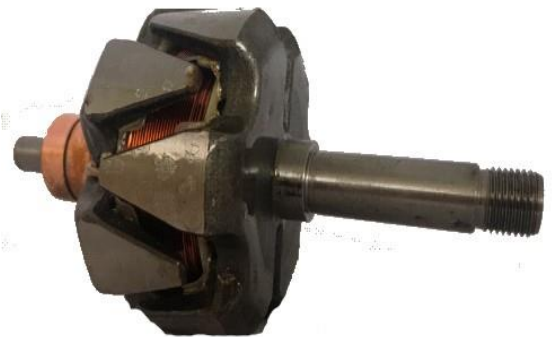
ROTOR 1124034642 12V 55AMP ADE SMALL ROTOR
